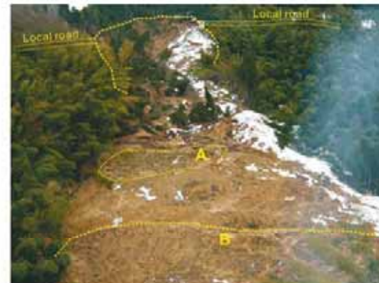
Fig. 8 Air photo of the second flowslide occurred on December 31, 2003 (taken with remote-controlled camera in balloon, photo courtesy of Agriculture and Forestry Central Administration Office, Ishikawa Prefecture). (A) The grass previously distributed in the apple yard behind the main scarp of the first flowslide. It moved for 200 m as a whole block. (B) Deposit of the first flowslide. It bulged up because of the pushing by the second flowslide.
