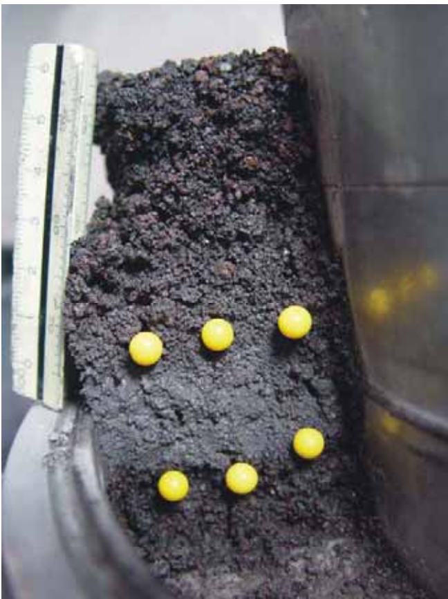
Fig. 11 View of the shear zone after the test
