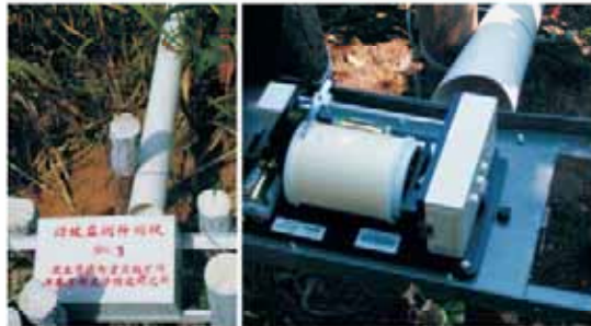
Fig. 40.8. Extensometer installed in Shuping landslide. The deformation is recorded on the rolled paper and also saved in a memory (visible in the right side)
