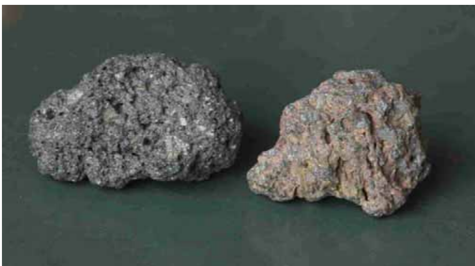
Fig. 5 Macrophotograph of black (on the left) and reddish (on the right) scoriae.
