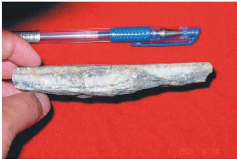
Fig. 11 Photograph of a crystalline calcite sample taken from the sliding surface at the upper part (the white color is crystalline calcite)
