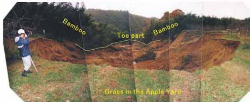
Fig. 2 Photograph of the first flowslide occurred on November 8, 2002 in Yamashina area (photo courtesy of Agriculture and Forestry Central Administration office, Ishikawa prefecture)
