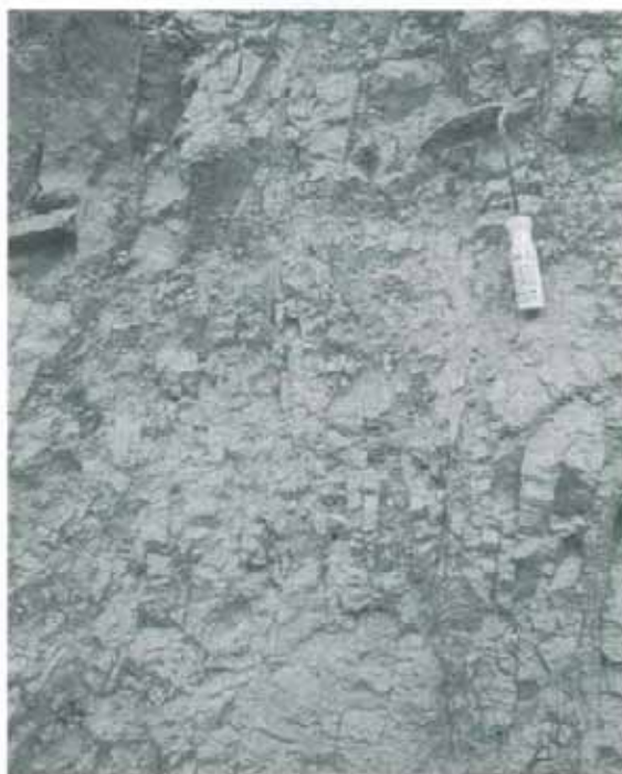
写真-5 滑落崖での風化泥岩の亀裂状況 Photo 5 The crack situation of the moderately weathered mudstone at the main scarp
