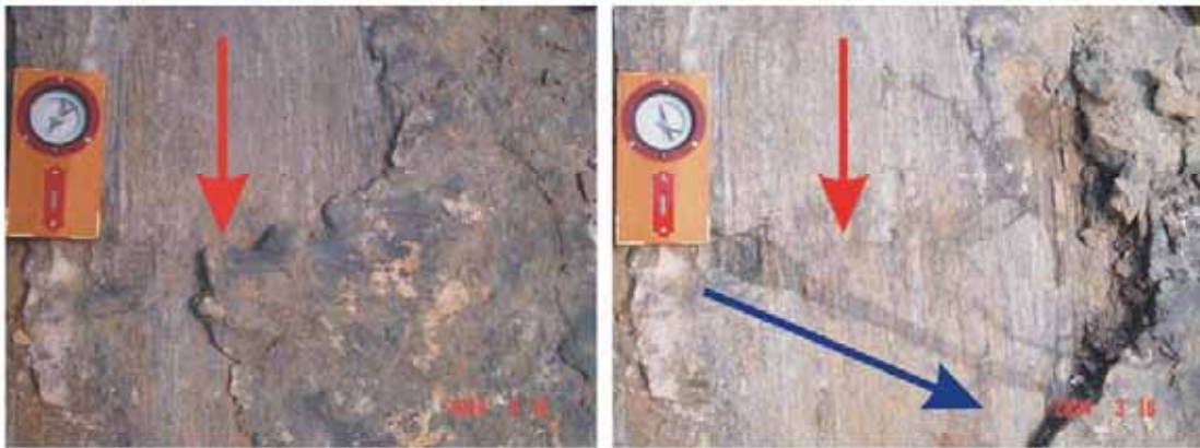
Fig. 8 A pair of photographs at the site showing the pre-existing scratches that underlie the sliding surface of the July 2003 event (blue arrow shows the sliding direction, red arrows show the strike direction of the pre-existing
