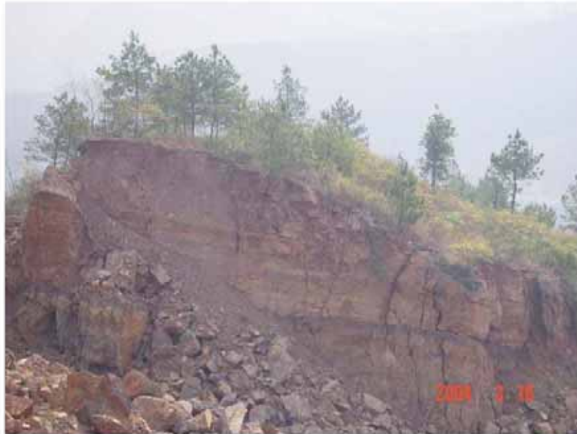
Fig. 4 View of the unrotated trees on the sliding mass in the middle of the Qianjiangping landslide
