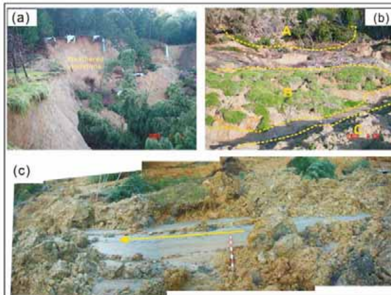
Fig. 9 Photographs showing the details of the second flowslide in Yamashina area. a The main scarp of the second flowslide (taken on January 1, 2004). b The toe part of the second flowslide. Part A shows the standing trees and bamboos; Part B shows the grass ground moved as a whole block; Part C shows the deposits of the first flowslide was pushed and bulged up. c The fresh mudstone outcropped as a sliding surface after the second flowslide
